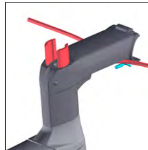
Install stem and steerer inserts
