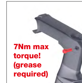
Install stem steerer clamp bolt - grease required!
