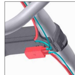
Install Di2 junction box (optional)
