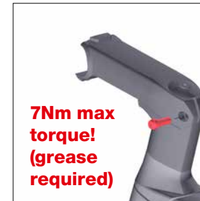
Install stem steerer clamp bolt - grease required!
