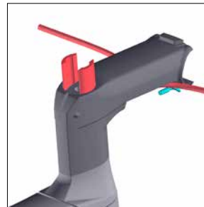
Install stem and steerer inserts
